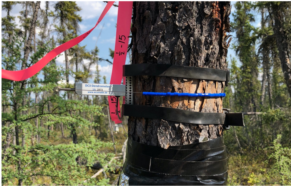
Figure 1.7 A dendrometer installed on a black spruce at Smith Creek. Photo: Nia Perron.
