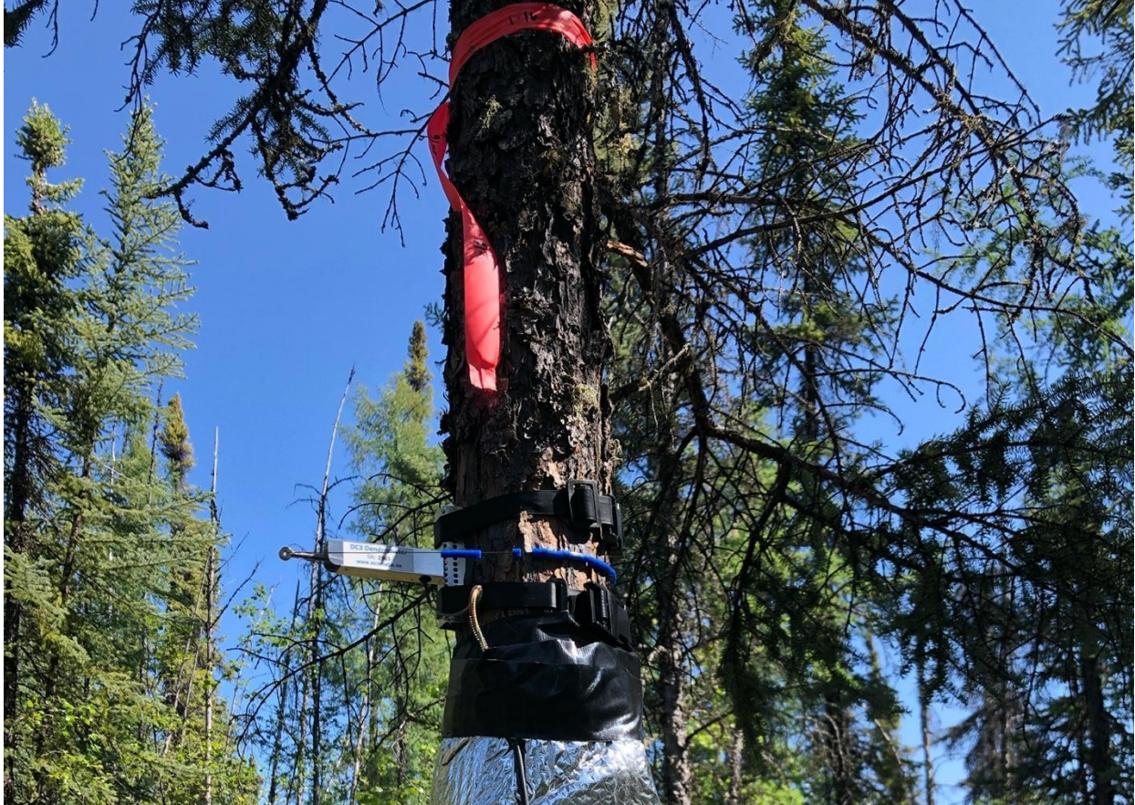
Figure SI.1 : A dendrometer installed on the stem of a black spruce tree at Scotty Creek (SCC).
