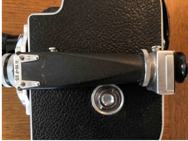
Bolex H16 clear trifocal viewfinder. See database entry.
