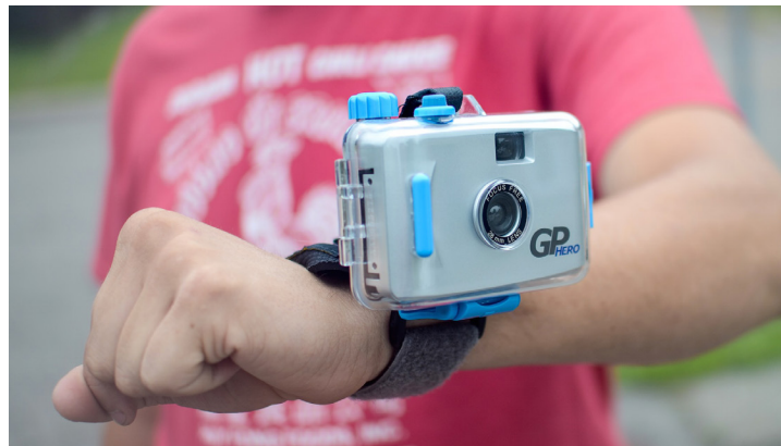
35 mm GoPro HERO film camera with its waterproof case and integrated mounting strap. See database entry.
