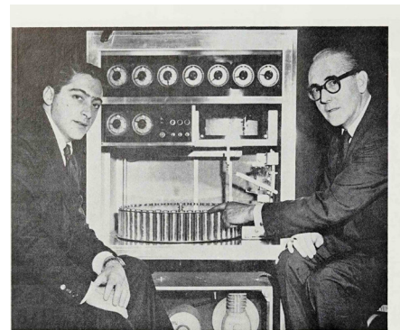
THE BRAINS OF SMELL-O-VISION—Michael Todd, Jr. (left) sits beside master control and scent energizer of the Smell-O-Vision system with its inventor Hans Laube. Latter points to the multitude of vials each containing a different scent which is selectively projected through tubes to every seat in theatre on signal triggered from picture's sound track.
