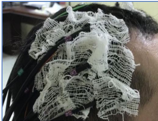
Figure 23 – Multiple optodes installed using gauzes impregnated with collodion on a subject in our lab.
