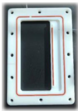
Figure 2.5 – The Teflon insert serving as the centre of the reactor.
