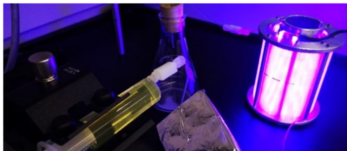
Figure 4.4 Scale-up of the photochemical E \leftrightarrow Z isomerization using continuous flow methods.
