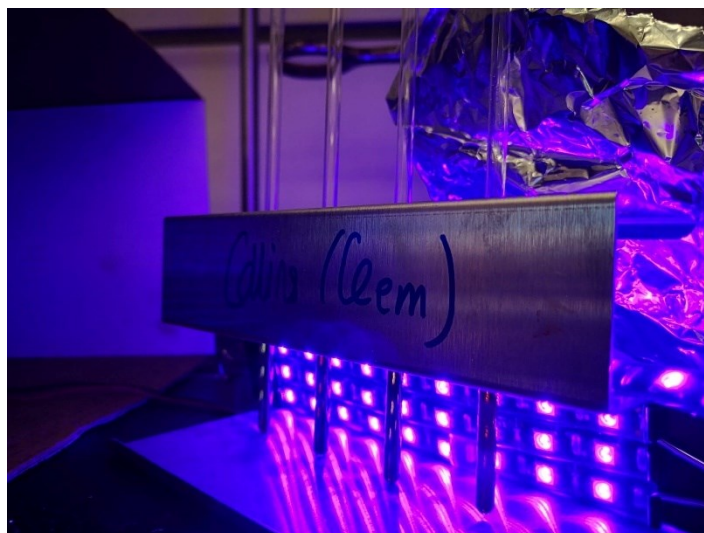
Figure A3 - 43 Setup for the photostability of copper complexes
