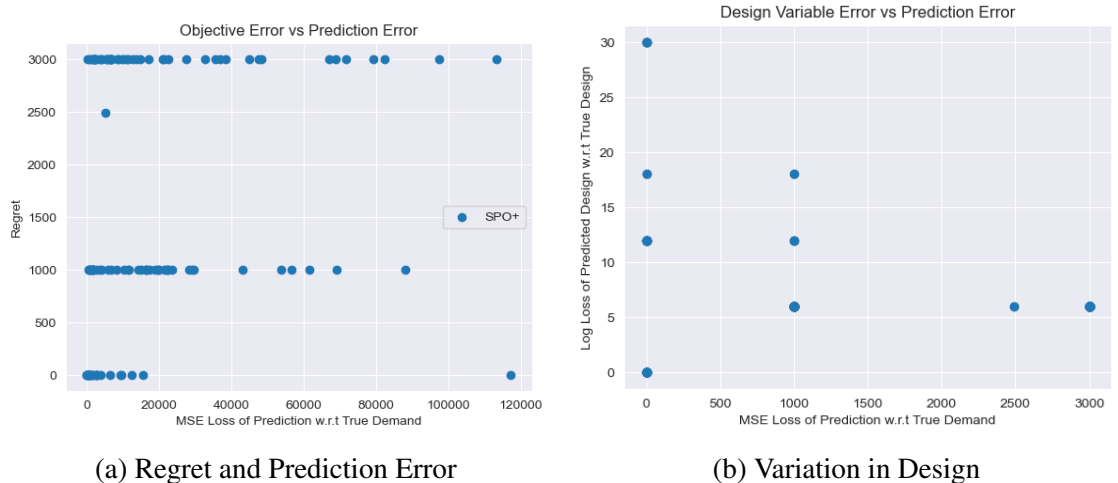
Figure 4.10 – Objective and Design Graphs for Scenario 3, SPO - The left graph shows the relationship between Regret and MSE Prediction Error. The right graph shows the relationship between the difference in design variable selection and MSE prediction error.
