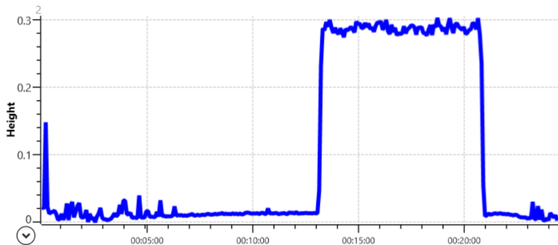
Concentration profile of the 1183 cm -1 band (B-F stretch) over time (min)
