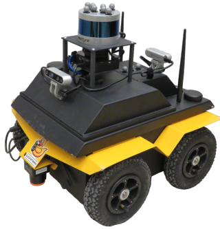
Fig. 4.8. We use the Jackal UGV mobile platform [118] using the RGB channels (no depth) of two Realsense D435i cameras with a 90^\circ FOV. We detect forward collisions using a forward-facing Hokuyo laser scanner. We run O4A onboard using an Intel i7-8700 CPU with 32 GB of RAM. We did not require a GPU for navigation.
