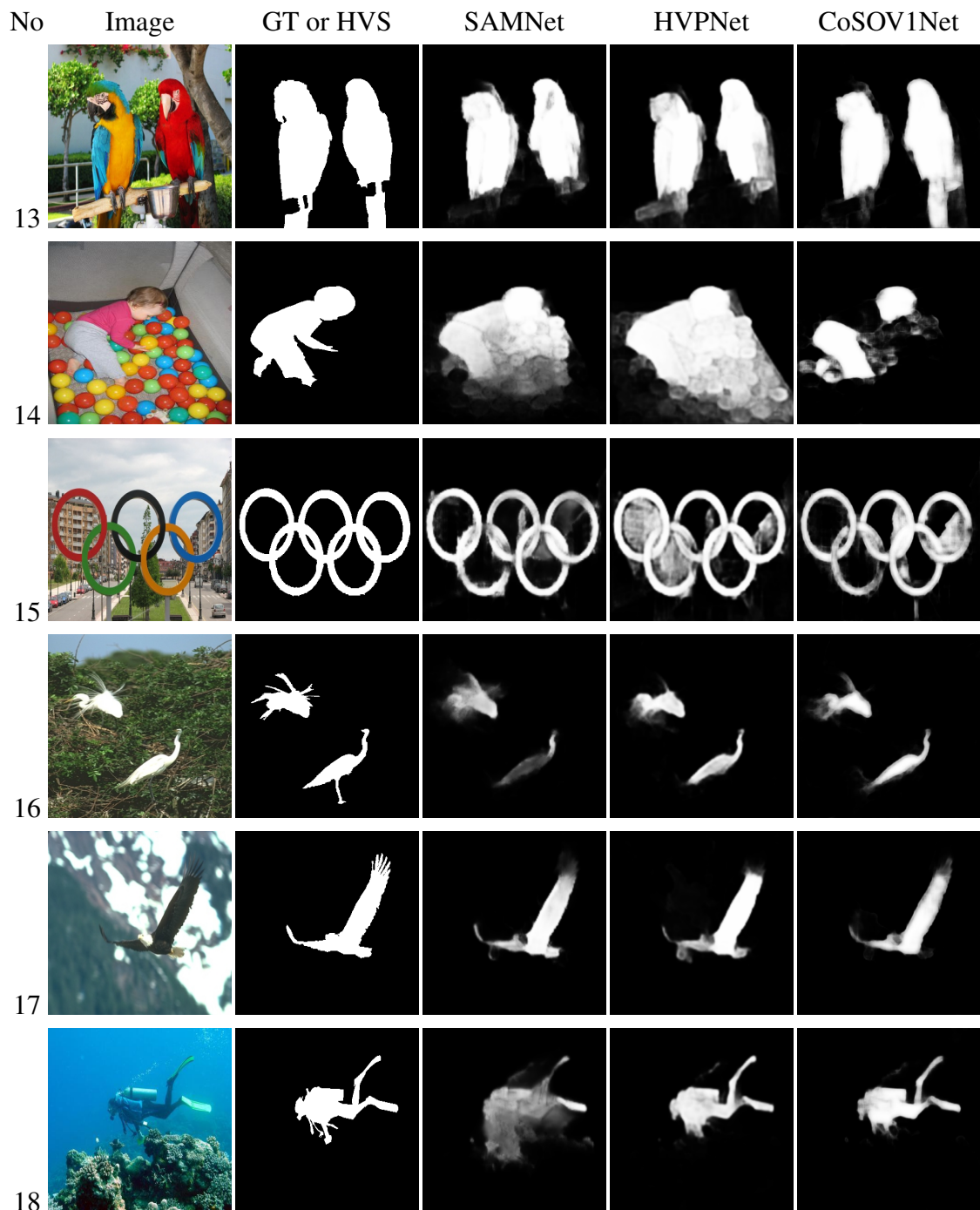
FIGURE 5.11 : Comparison between SAMNet [16], HVPNet [19] and our proposed model, CoSOV1Net, on some image saliency maps : 1st column : images ; 2nd column : ground truth or human visual system saliency map ; 3rd column : SAMNet ; 4th column : HVPNet ; 5th column : CoSOV1Net (ours).
