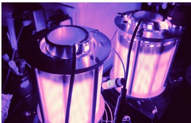
Figure 4.4 : Experimental set-up for the photocatalytic conversion of alcohols to bromides. PFA tubing is wrapped around purple LEDs (394 nm) and fans are placed underneath reactors to maintain cooling
