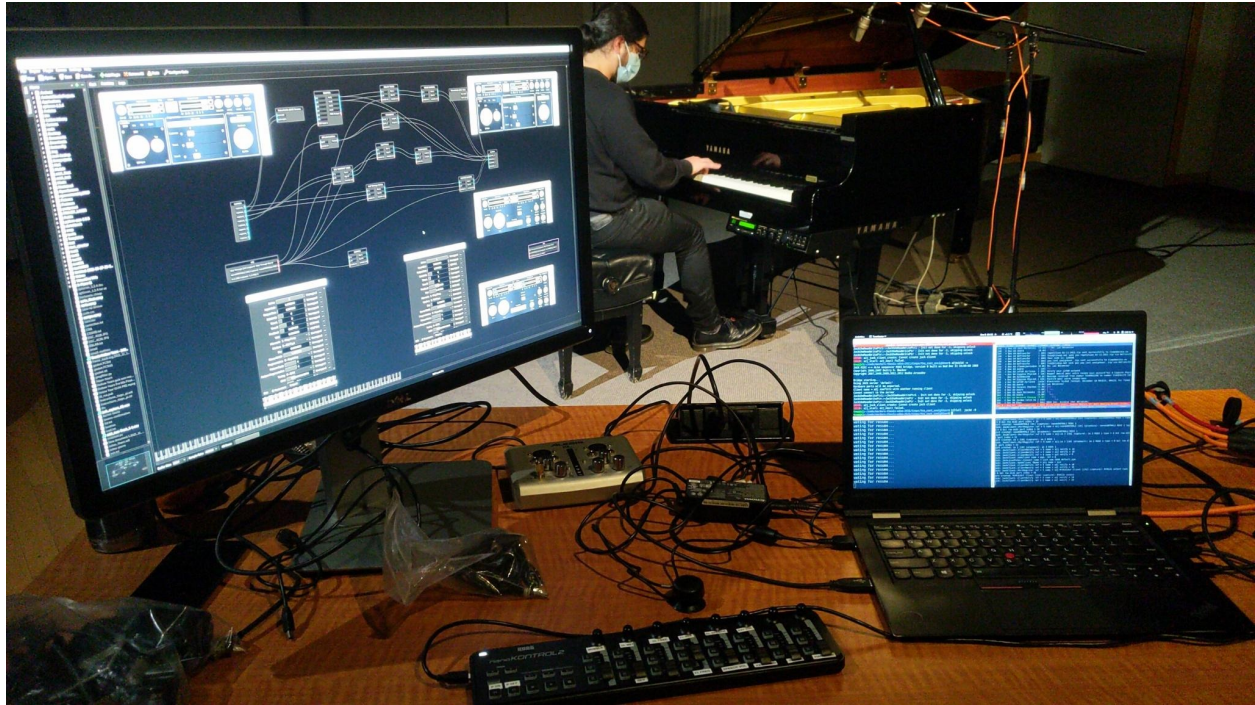
Figure 3.15. Live electronics setup using Carla, Pyo and a MIDI controller in You can't un-neighbor your neighbor .
