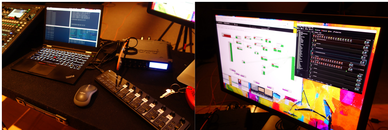
Figure 3.13. Live electronics setup using Carla, Jack, Pyo and a MIDI controller in “You’re thinking I’m a good person”.
