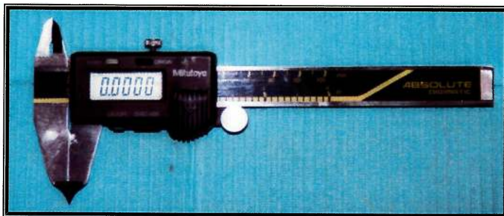
Figure 9.1 : MITUTOYO Absolute Digimatic (jauge digitale)
