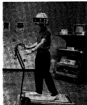
Example of an early input device for an architectural "walk-through" application. The user walked on a treadmill that helped generate the illusion of strolling through the virtual building seen on the head-mounted display. The treadmill recorded the direction (using handlebars) and extent of the user's walking. Distance walked in the virtual world was matched to distance walked on the treadmill. Courtesy of the Computer Science Dept., University of North Carolina at Chapel Hill.
