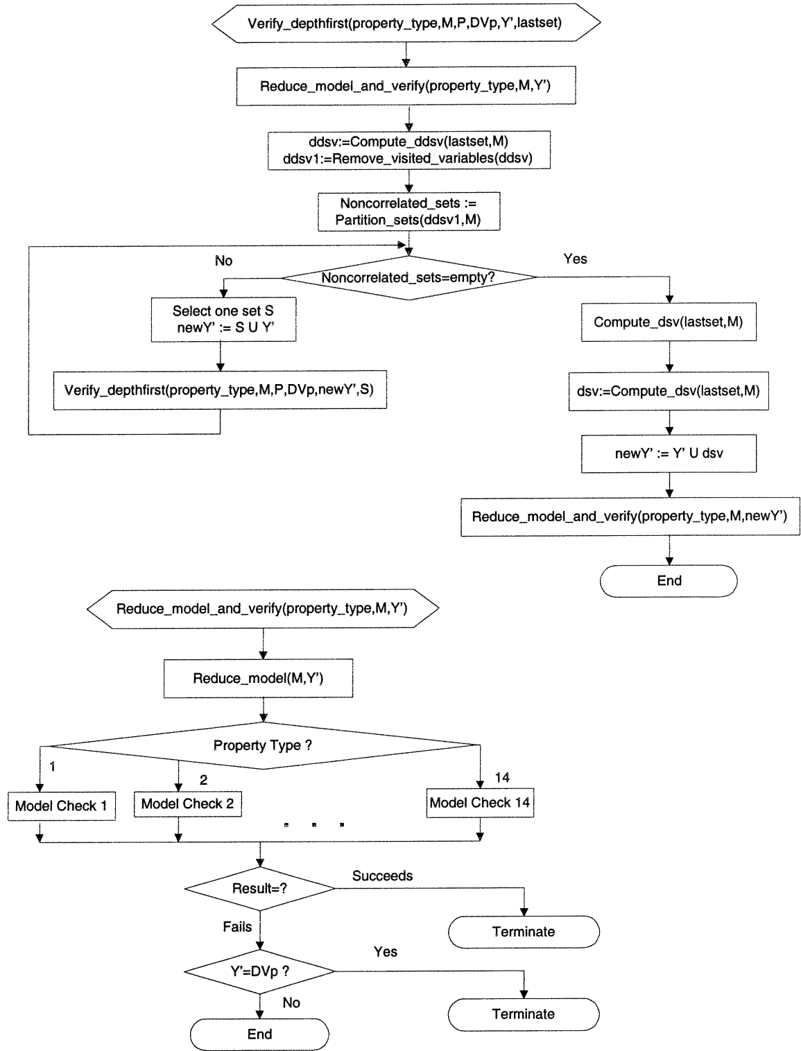
Figure 22. Flow chart of procedure Verify_depthfirst in MDG model checker
