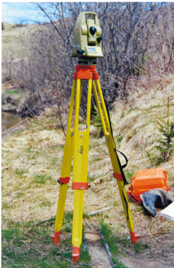
Figure 2.3: Station totale Leica TC805L.
