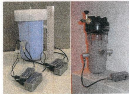
Fig. 1. Two large-volume droplet detectors. On the left is a 3-liter volume unit; the one on the right has a 1.5 liter volume (10 cm width). Containers can hold pressures up to 150  $lb/in^2$ ; piezo-sensors are glued on the containers.
