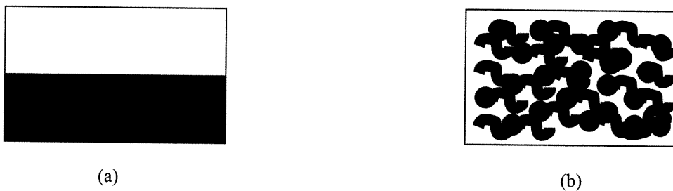
Figure 1.6 Conceptual sketch of (a) total phase separation and (b) microphase separation for a mixture of two components, in this case, polymer network and water. (b) is often the result of spinodal decomposition. The dark region corresponds to the polymer phase and the white region corresponds to the water phase.
