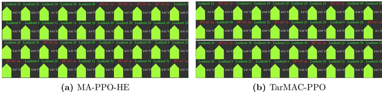
**Fig. 4.** State of 20 houses controlled with two different PPO agents. The number on the top right is the remaining lockout time. (Left) Two different agents of MA-PPO-HE with  $N_{c_{de}} = 19$  show a “20-house” (up) and a “3-house” (down) pattern. (Right) Two different TarMAC-PPO agents show no such pattern.
