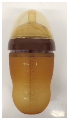
Figure 24. Piko Bello baby feeding bottles coated with silver nanoparticles. The surface area of contact is 707 cm 2 . Containers were purchased from DHgate.com (China).
