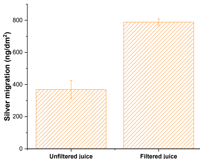
Figure 20. Migration of silver from the Rubbermaid containers into (a) filtered and (b) unfiltered orange juice after 4 days. Analysis performed using single particle ICP-MS.
