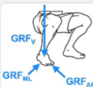
Figure 1: Ground reaction forces in the vertical (GRF v ), antero-posterior (GRF AP ) and medio-lateral (GRF ML ) directions.
