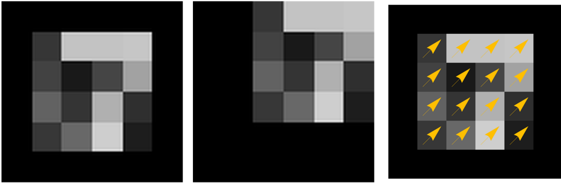
Figure 1.1: Optical flow estimation. A grid of instantaneous motion vectors is computed from a sequence of images. Left: I_1 and I_2 , Right: I_1 's optical flow.
