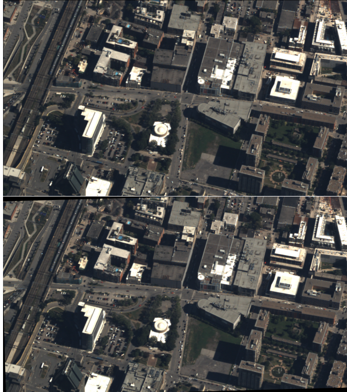
Figure 3.9: Aerial stereo pair. Notice that the second image has been rectified to align its epipolar geometry.
