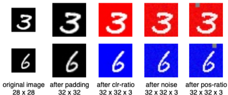
Fig. 3.1. The conversion process used to generate samples. Input image is first padded to become 32x32. The attributes clr-ratio is then applied, which decides the background color (blue or red). Noise is then added to the background color. Finally, pos-ratio affects the positioning of the box (top row, left half or top row, right half).
