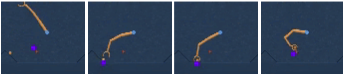
Fig. 8.12. Qualitative Evaluations. Model leverages object centric representation model to learn the object keypoint. The inferred object location is used to compute the intrinsic reward inorder to solve the bring ball task.
