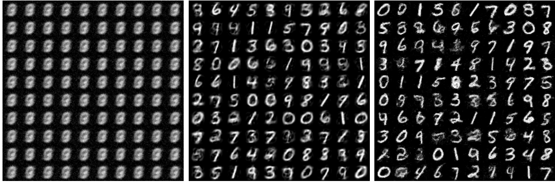
Figure 4.6: All 100 Prototypes learned using linear ( left ), dense ( middle ), and CNN discriminator ( right ). We observe that with the linear discriminator, only the mean of the training set is learned, while using the dense discriminator yields blurry prototypes. Only the CNN discriminator yields clear prototypes.
