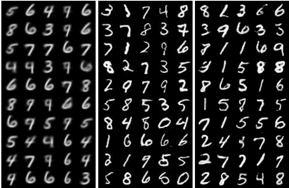
Figure A.4: Samples from generators with similar architecture and 200 latent variables, trained with the following objectives: VAE ( left ), WGAN-GP ( middle ), and WGAN-GP with side-task ( right ). Each row represents a sample (combination of 5 digits) generated by the model.
