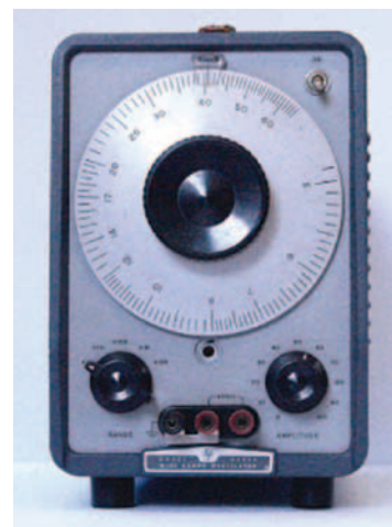
Fig. 1. One of the analog oscillators used by Ensemble d'oscillateurs: a Hewlett-Packard 200CD oscillator, generating signals from 5 to 60 cycles per second in five ranges, 2018. (Photo © Nicolas Bernier)
