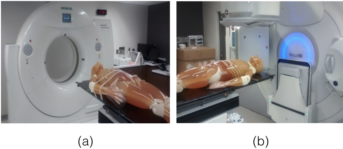
Fig. 8.1. An anthropomorphic phantom laid down on the rotating table for acquisitions by CT on rails (a) and on-board cone-beam CT (b).
