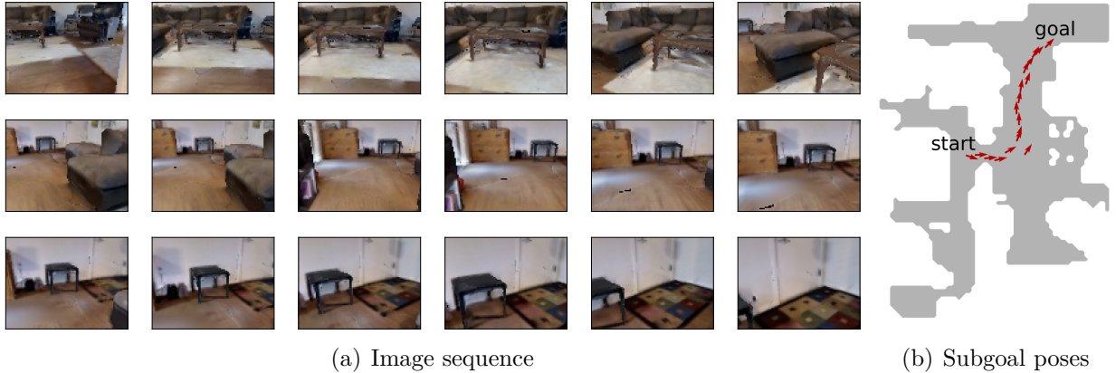
Figure 1.1. A sample plan produced with our method to move from the top-left to the bottom-right image. The intermediary subgoal images transition smoothly, which helps the robot’s image-based controller easily navigate to the goal.
