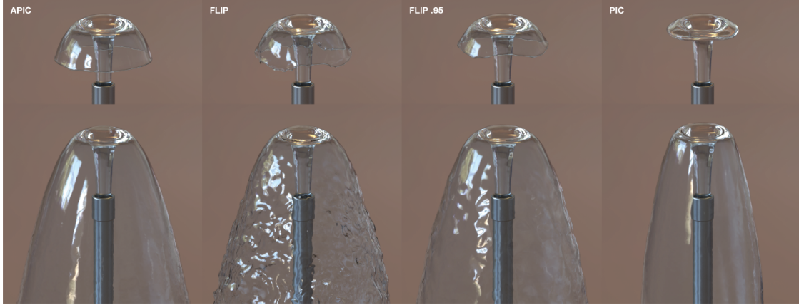
Figure 1.5. Comparing Affine-PIC (APIC), FLIP , PIC-FLIP , and PIC . The APIC method considerably reduces the noise generated by FLIP while preserving the nature of the fluid [17].
