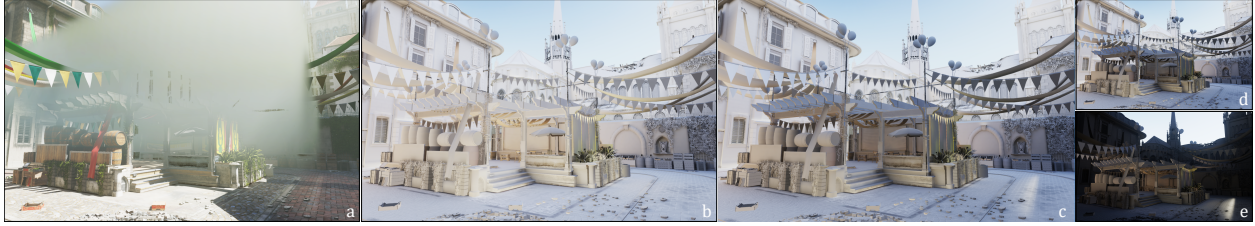
Fig. 19. In-game screenshot (a) with complex surface and volume shading. Standard lightmaps (b) ignore volume-to-surface transport, which our method compensates for (c) with media-attenuated surface global illumination (d) and volumetric single- and multiple-scattering (e).
