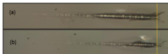
Fig. 5. Optical microscope pictures of micro-scratch performed on coatings (a) Low Pressure (b) Atmospheric Pressure. Maximum load of 15N (orange dashes).
