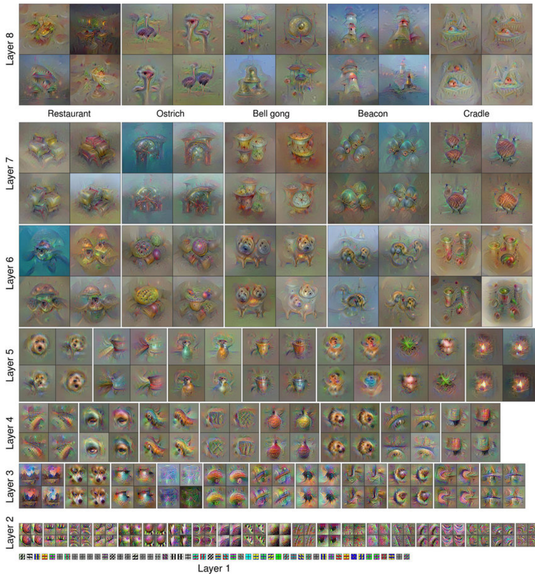
Fig. 1.5. Use of multifaceted feature visualization to show what each layer of a Convolutional Neural Network learns [78]. Each pixel of each picture corresponds to a single neuron in the network.
