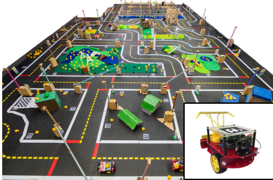
Fig. 5.1. The Duckietown Autolab: We augment Duckietowns [64] with localization and automatic charging infrastructure. We modify Duckiebots (inset) to facilitate detection by the localization system and auto-charging.
