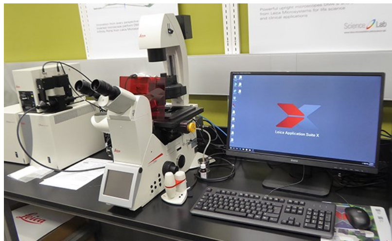
Figure 8. – Leica DMI-8 wide-field microscope. A 10X objective with a 1X magnification was used for the imaging of the specimen for each experimental condition.
