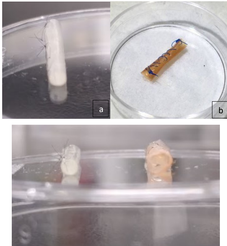
Figure 2. – Hollow conduit without silk PEM (a) and Hollow conduit with silk PEM (b). Both conduits were made from 15 x 20 mm pieces of collagen sheet (a) or collagen coated with silk PEM (b).
