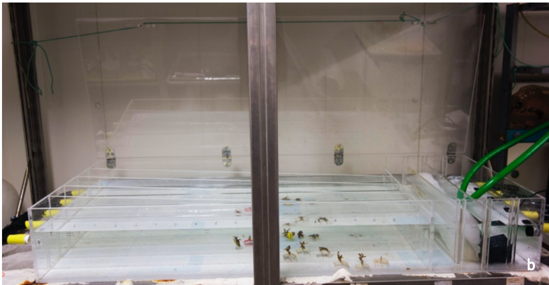
Fig. 3. a, A drawing and b, Photograph of the experimental aquarium with flow channels. One channel was used for control, with 0 cm/s flow, and three channels were maintained at flow velocities of 1.6 cm/s, 2 cm/s, and 3.3 cm/s. In figure a, arrows indicate the direction of flow, and velocities in cm/s are reported on each channel.
