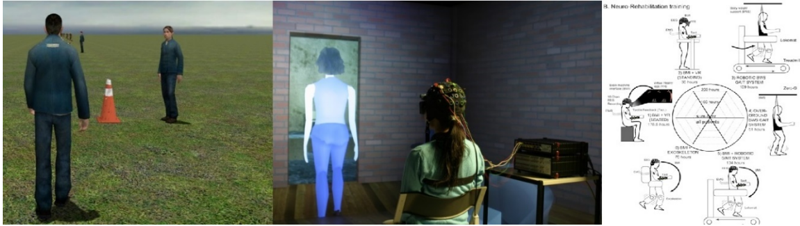
Figure 1.13 BCI systems to control an avatar: An avatar controlled by a self-paced BCI (left) [3], a female participant controlling the gait of her avatar in the virtual room (middle) [40], control of the right/left steps of an avatar, then of an exoskeleton with a BCI (right) [55]
