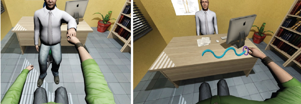
Figure 1.18 Person-to-person haptic interaction with force feedback in VR. The remote doctor explores patient's arm mobility. The patient sees a virtual representation of the real doctor, which gives the hand to him (left). The ring task. A virtual ring is passed along a virtual wire without touching it. Whenever the wire is touched, force-feedback is enabled. Camera view is from IPP(right) [238]
