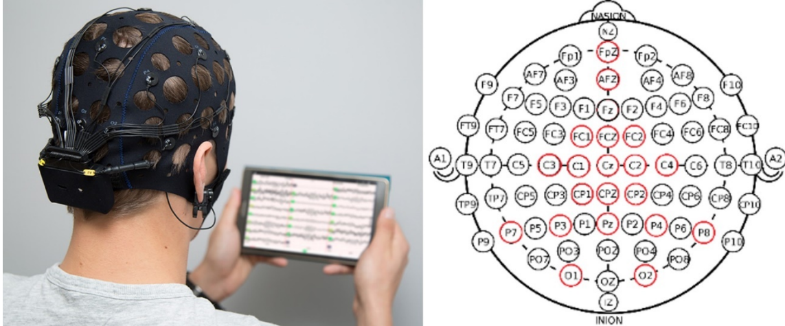
Figure 3.5 The Smart BCI system (left) EEG-electrode configuration used for this project (right).
