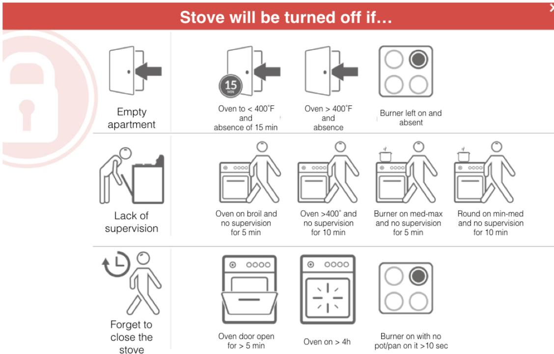
**Figure 3. Rules of the Self-monitoring Security System (SSS)**
