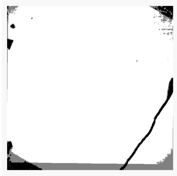
Figure S9 - Mean image for the image registration of an untreated zone and the same zone after plasma treatment. A criterion based on the G-band intensity is used to distinguish between specific zones within the graphene sample. Defects are therefore aligned so as to allow point by point analysis. Two mask of logical values are aligned. Points where both signal are 1 appear black; points where both signal are 0 appear white and points which values are opposite appear as grey.
