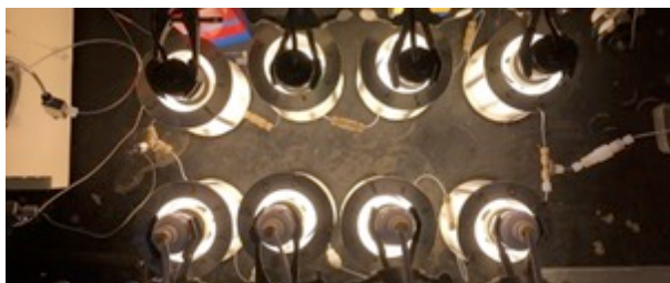
Scheme 2.3 Numbering up strategy for the gram-scale synthesis of carbazole 2.2 : synthesis of simple and complex carbazoles.
