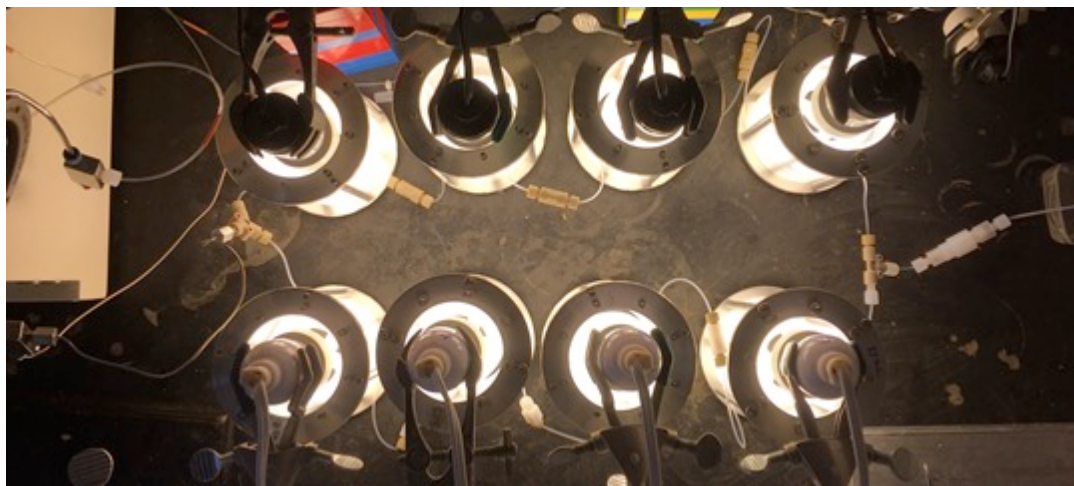
Figure 6.3 Continuous-flow reactor numbering-up set-up used for the visible light mediated synthesis of carbazoles.
