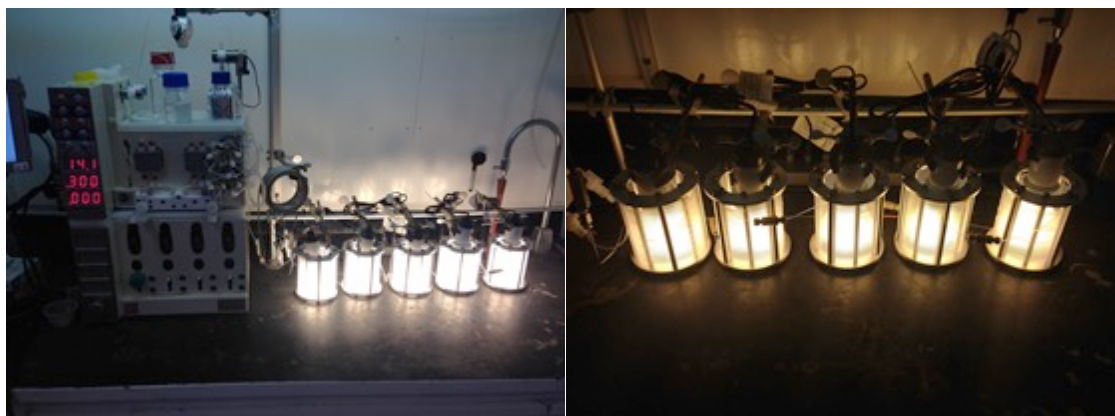
Figure 6.1 Continuous-flow reactor set-up used for the visible light mediated synthesis of carbazoles. (left: VapourTec module connected to five PFA coils; right: disposition of CFL inside PFA coils)
