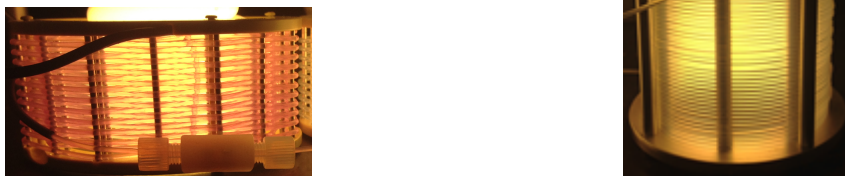
Figure 6.2 Continuous-flow reactor. (left: Vapourtec PFA coil (10 mL, 1 mm I.D.) ; right: homemade PFA coil (12 mL, 1 mm I.D.)
