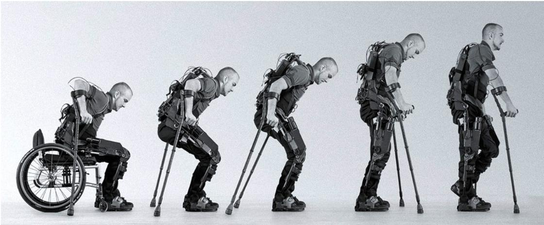
**Figure 4.** – The WRE enables standing, sit-to-stand transitions, and overground walking.
