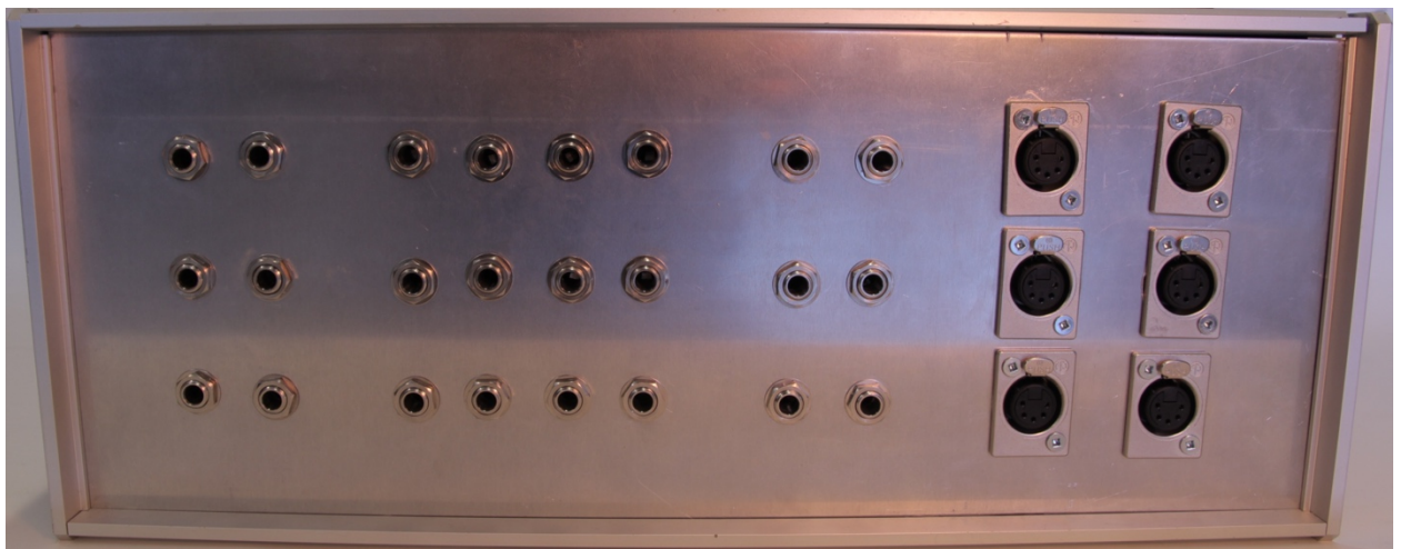
Figure 17: Master spring control box, including inputs for foot pedals and carabiner buttons, and outputs for electromagnets and 100W LED lamps.
