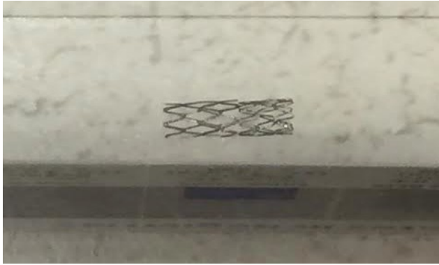
Figure 7. Plasticised bare-metal cobalt-chromium stent. With permission from Hôtel-
