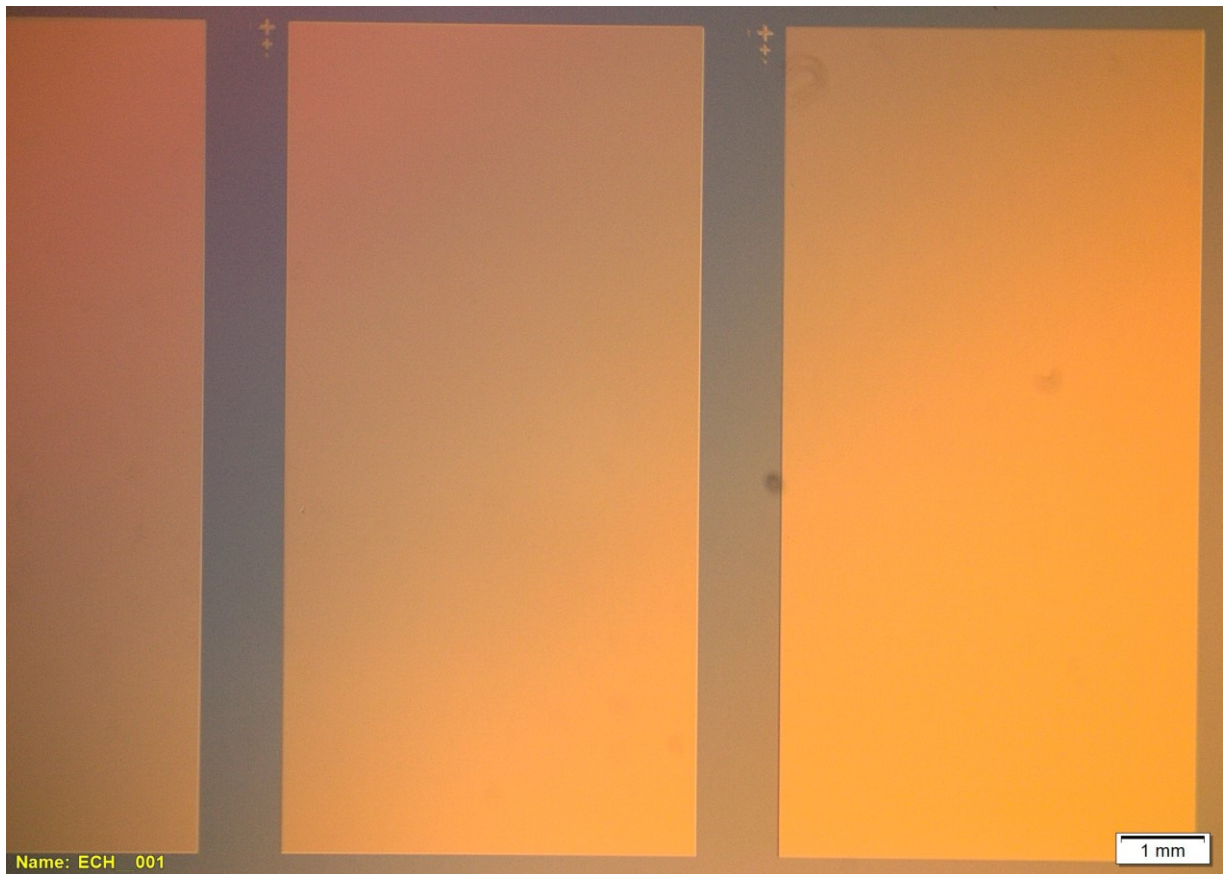
Figure D.1: bottom electrode (ground) deposited by E-beam
