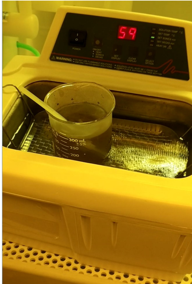
Figure 4.28: Bain Marie used for lift-off with ultrasound waves
