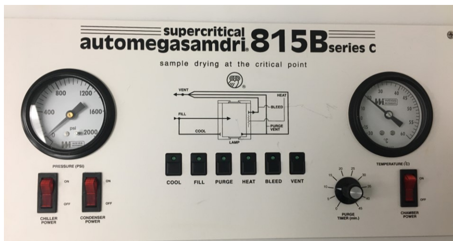
Figure 4.21: CPD control panel
