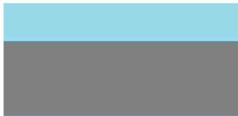
a) Growing silicon oxide on a silicon wafer
