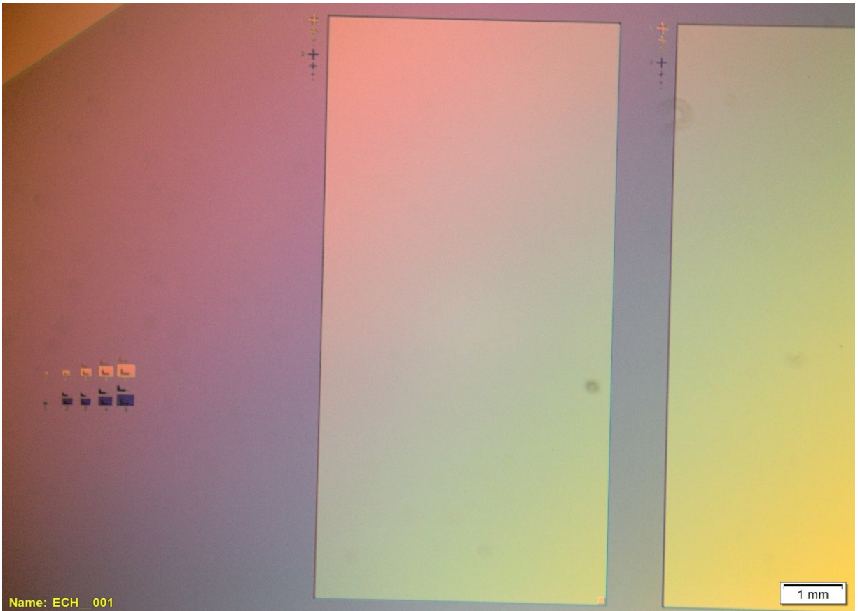
Figure D.2: transparent Si 3 N 4 insulation layer covers the bottom electrode
