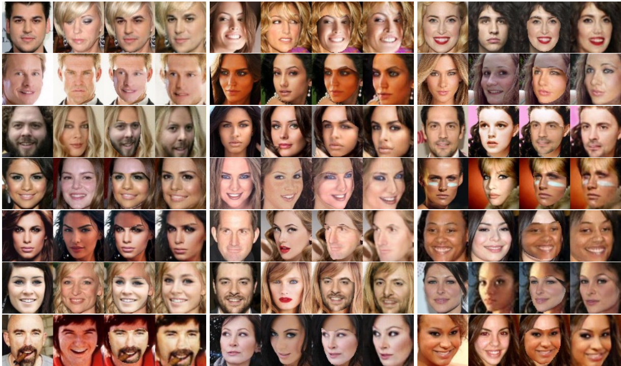
Fig. 10.10. Face swap experiment with CycleGAN. Left to right: source face; target face; warp to target with DepthNet; repaired result with CycleGAN. The source face is taken and warped onto the target face. The background and hairstyle is then adapted to the target face.
