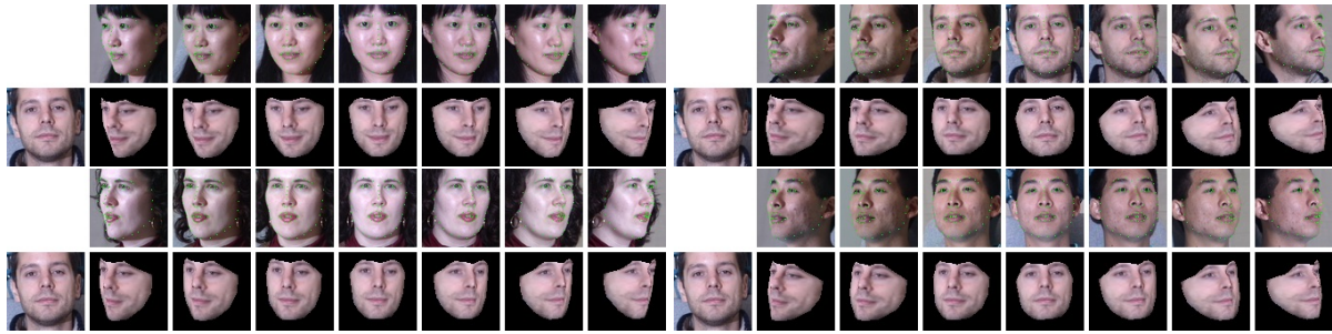
Fig. 10.6. Projecting a frontal face (far left) to a range of other poses defined by faces in the row above.
