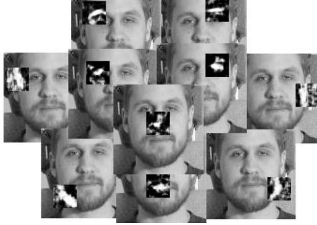
Fig. 4.2. Sample SVM response maps for an image generated by trained SVMs. Each response map is generated by one local classifier trained for a particular keypoint.
