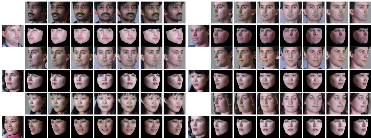
Fig. 10.7. Re-projecting a non-frontal face (far left) to a range of other poses defined by faces in the row above.
