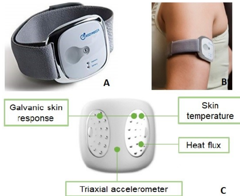
Figure 5-6. SenseWear Armband. A) Front view of the equipment; B) SenseWear Armband worn on the back of the arm; C) Back view of the equipment.
