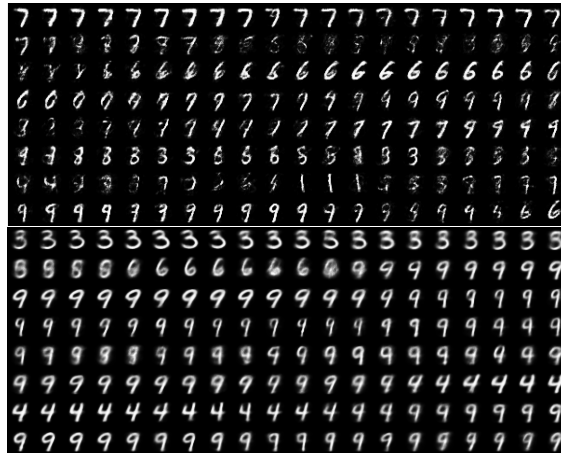
Figure 5.4 – Successive samples generated by Markov chain associated with the trained DAEs according to the plain sampling scheme (left) and walkback sampling scheme (right). There are less “spurious” samples with the walkback algorithm.
