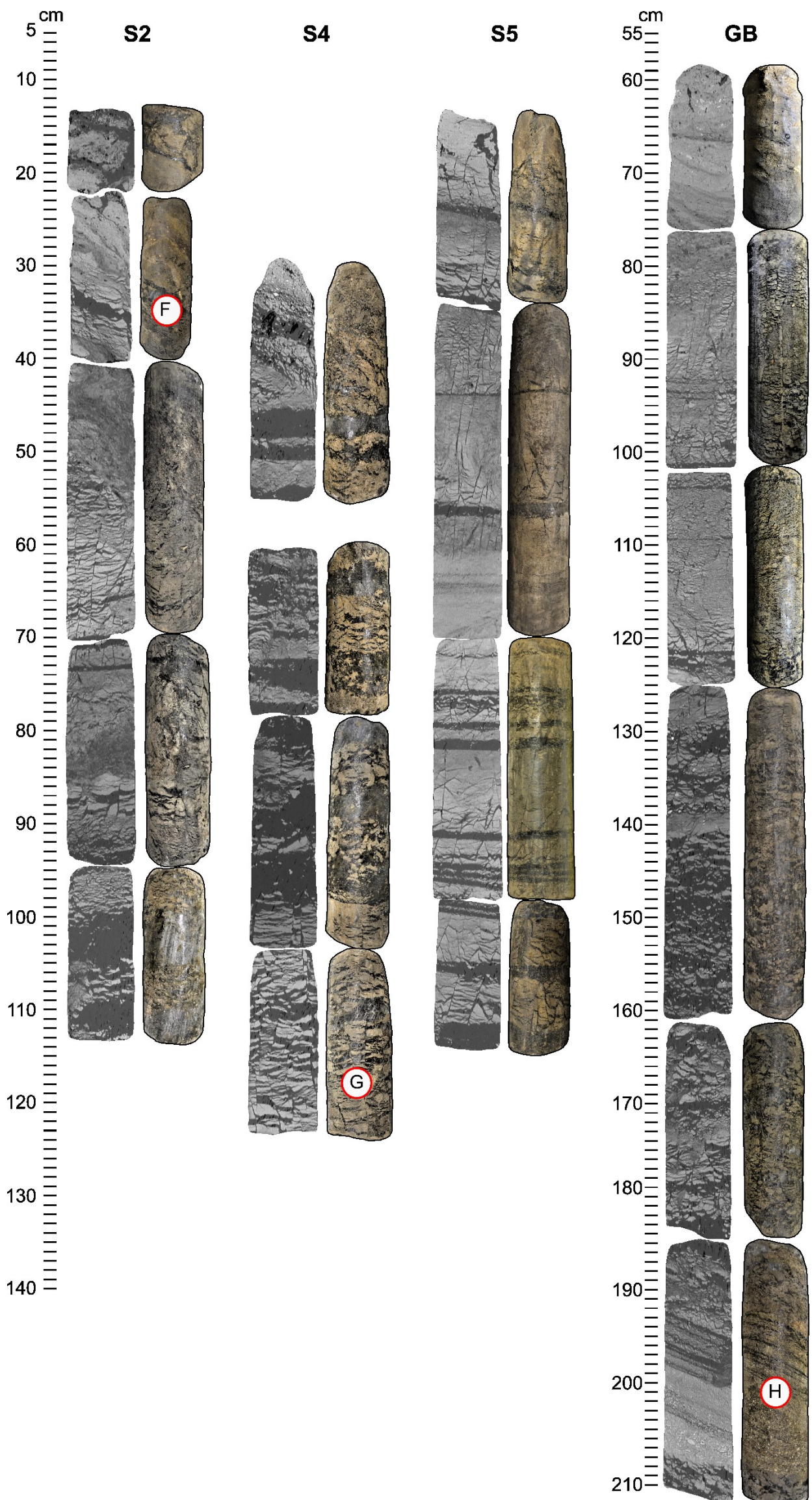
Annexe 3.1.1 Complete sequence of permafrost cores shown via CT-Scan imagery (left) and photographs (right) for the gully slopes (S2, S4 and S5) and the gully bottom (GB).
