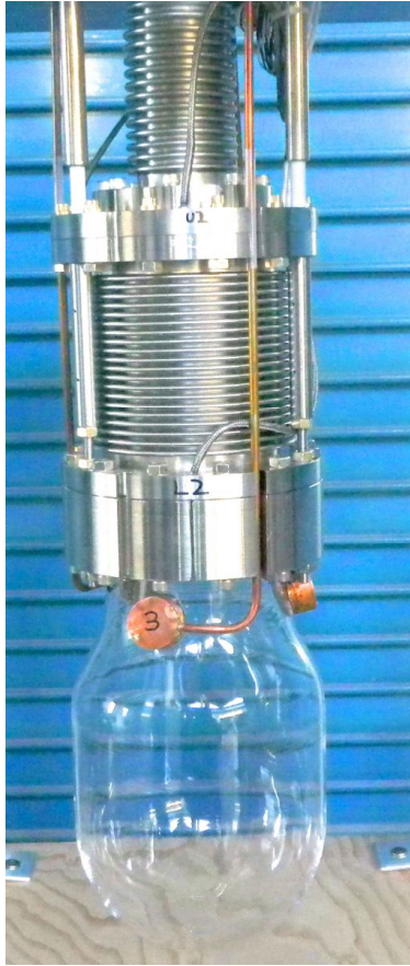
FIG. 4.6. PICO-2L inner vessel and bellows [21].
