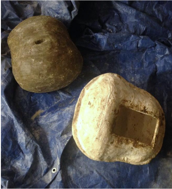
Figure 8.15. Slush cast mould and the final product (version 1).
